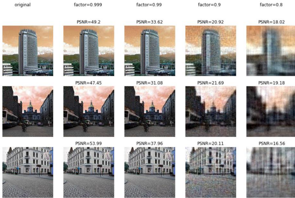
Figure 19: Performing PCA of an image with a given factor value representing the percent of variance to preserve. PSNR reflects the damage in image quality. The images are taken from the INTEL dataset.
