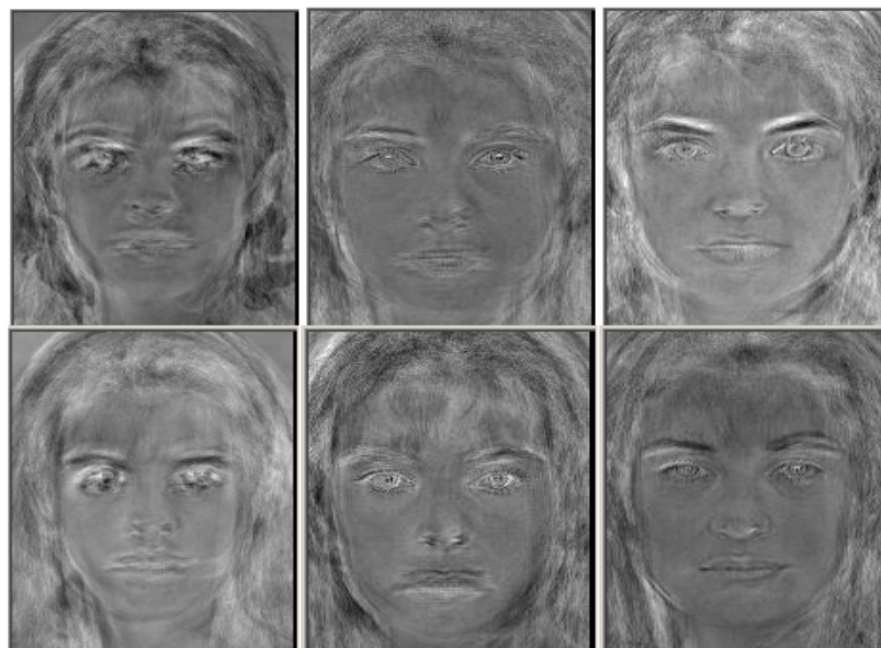
Figure 2: Left column: eigenfaces from unaligned images, middle: eigenfaces from images aligned only by eyes, right: eigenfaces from images aligned both by eyes and mouth.
